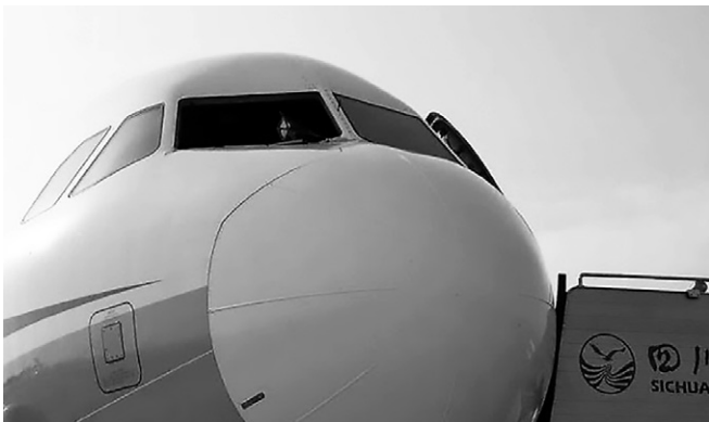
The Sichuan Airbus A319 lost his right windshield mid-flight.
