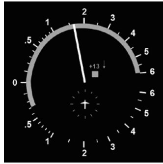
Fig. 7: A “level off” RA as depicted on a generic IVSI display.
