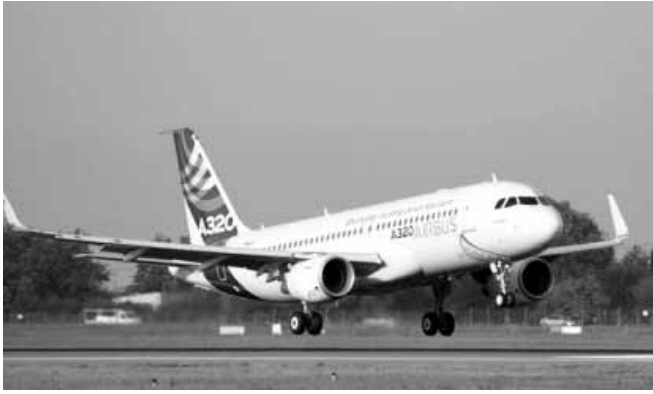
A modified A320 with sharklet wing tips.
