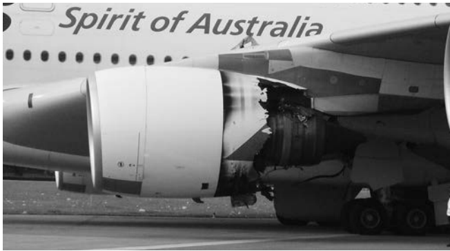
The Qantas A380 just after the uncontained engine failure.
