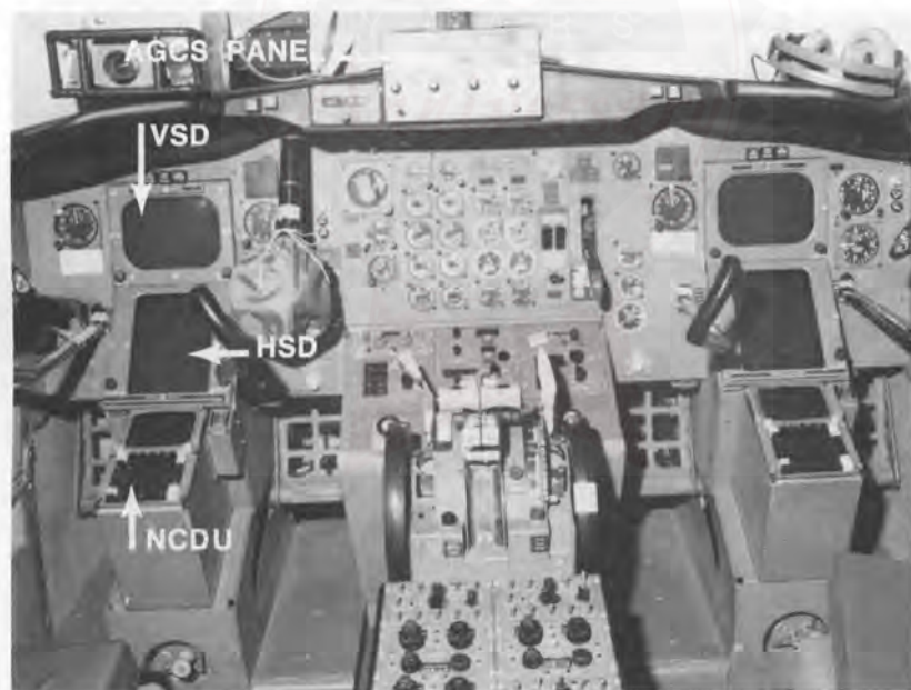
Fig. 2 AFD cockpit control and display layout
